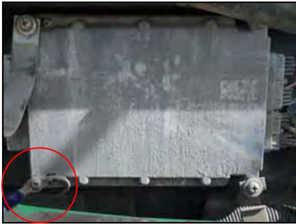
FIGURE 10. Node Harness Installed on Steering ECU
