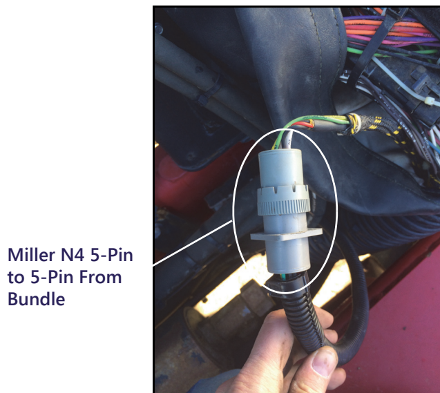
FIGURE 5. Miller N4 Interface Connected to 5-Pin Plug In Boot
