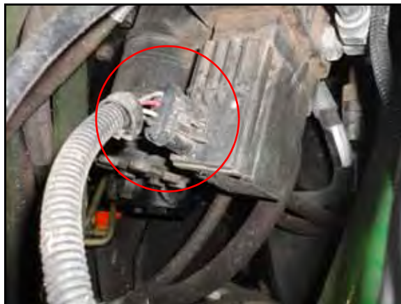
FIGURE 8. Machine's Existing Steering Valve Connection
