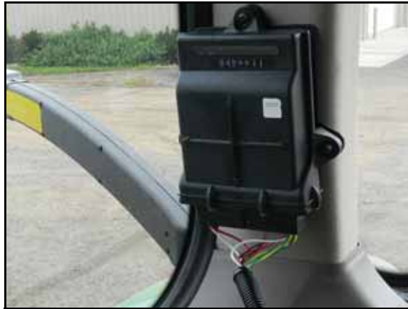
FIGURE 4. Node Cable Installed on Node
