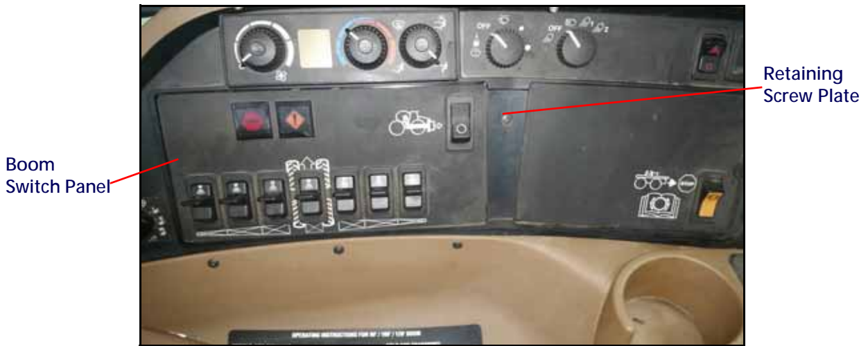
FIGURE 13. Switch Panel Access
