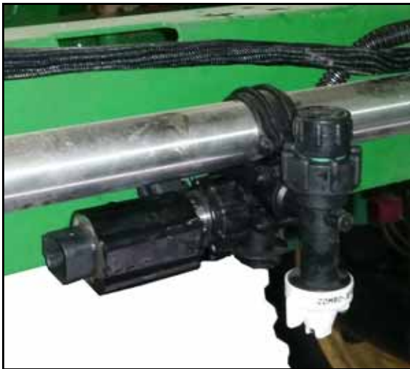
FIGURE 4. Wilger Nozzle Bodies Installed
