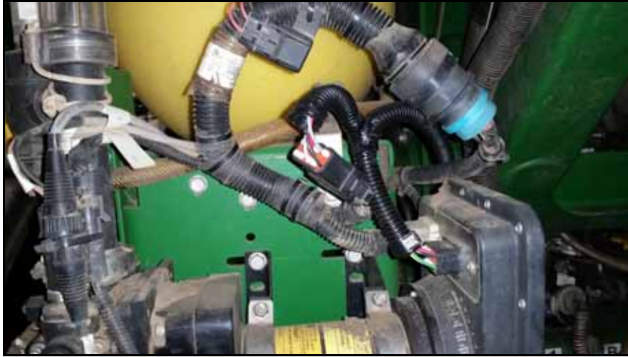
FIGURE 2. ICD Tee Cable Installed
