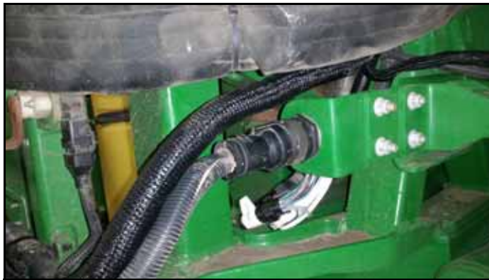
FIGURE 3. Connected Boom Cable
