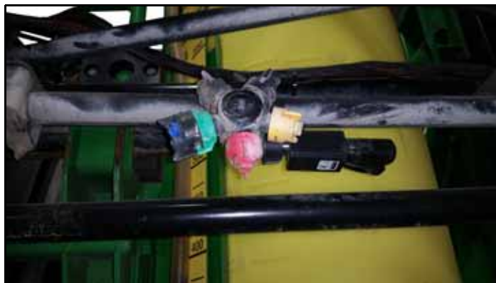
FIGURE 2. Installed Hawkeye Valve
