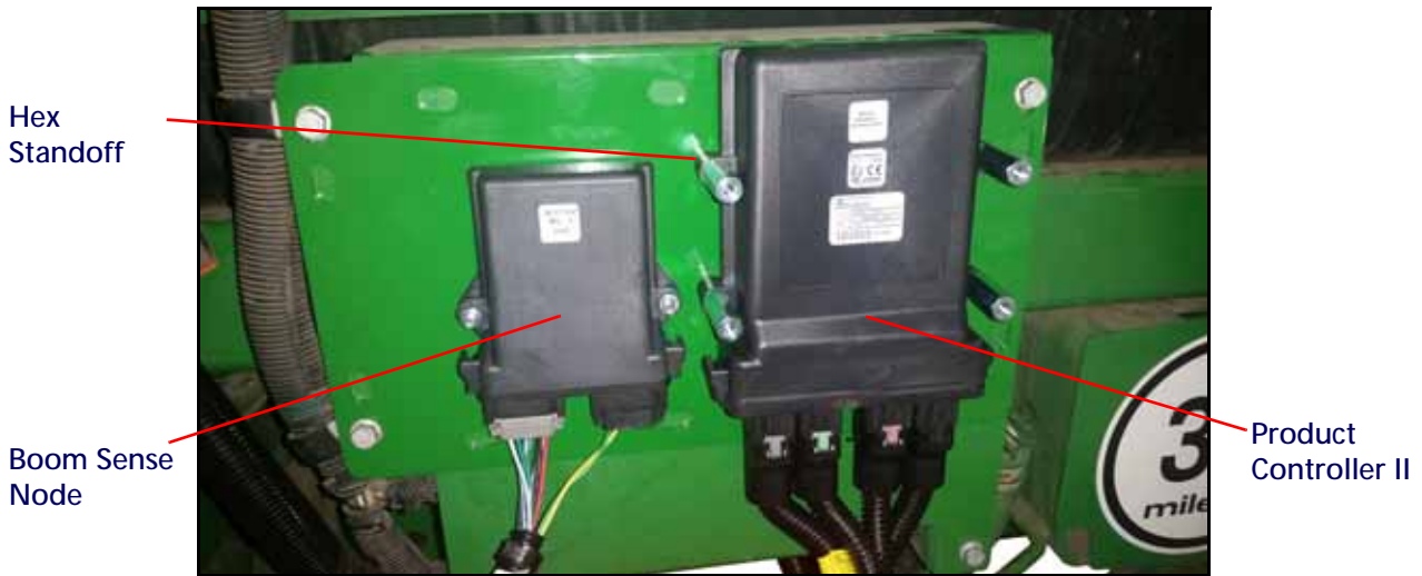
FIGURE 3. Installed PC II and BoomSense Node
