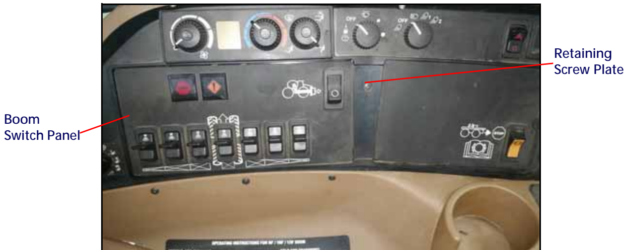
FIGURE 17. Switch Panel Access
