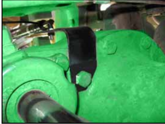
FIGURE 3. Base-End of Sensor Installed on Machine
