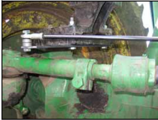
FIGURE 5. Rod-End of Sensor Installed on the Machine
