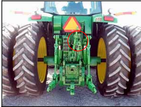
FIGURE 2. SmarTrax Valve Mounting Location
