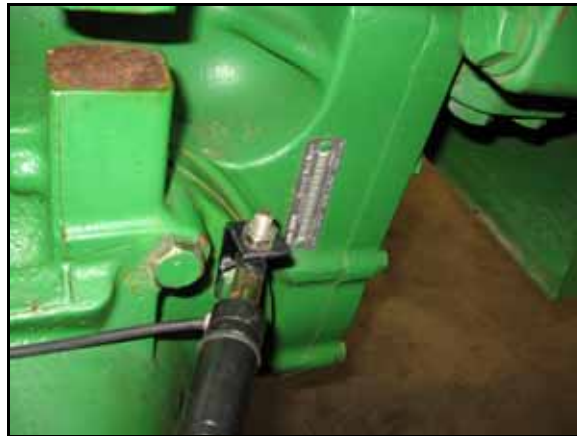
FIGURE 3. Base-End of Sensor Installed on Machine
