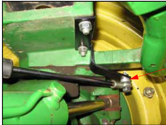
FIGURE 4. Rod-End of Sensor Installed on the Machine
