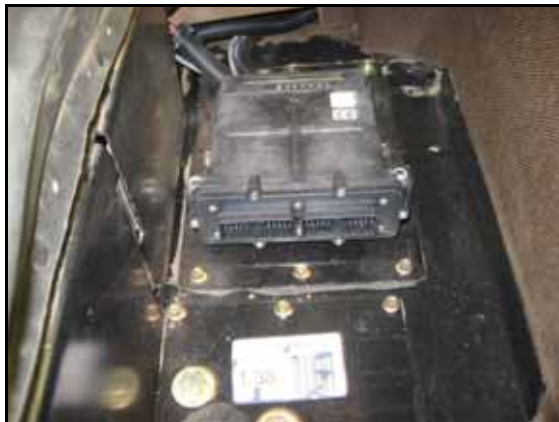
FIGURE 3. Node Installed on Node Mounting Plate
