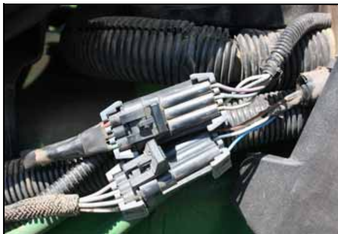
FIGURE 7. Wheel Angle Terminator
