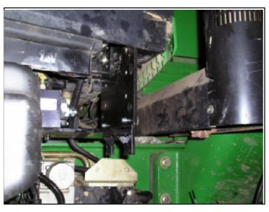
Attach pressure switch to PS port on SmarTrax valve before mounting valve.
