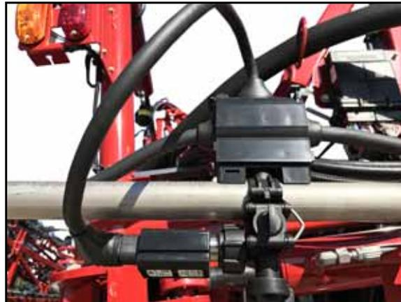
6. At each valve branch, adjust the cable as necessary to provide slack between nozzle control valve connections.
