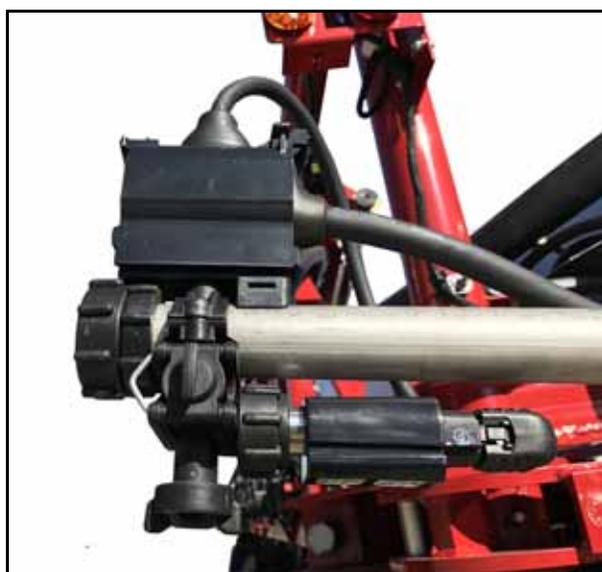
2. Use the provided hardware to install the harness mounting block.
