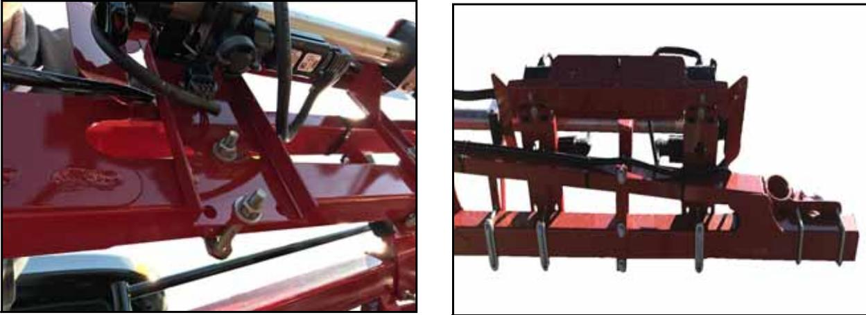
FIGURE 7. Nozzle Deflector Installation
