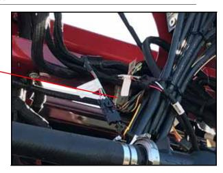
6. Route the connectors located "Left Boom" and "Right Boom" to the Primary AIM Command Flex nozzle cables installed in "Primary Boom Cable Routing and Connections" on page 15.
