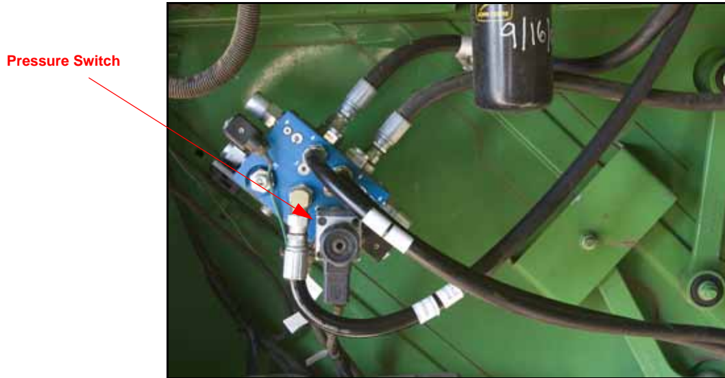
FIGURE 11. Pressure Switch Connected to SmarTrax Hydraulic Valve
