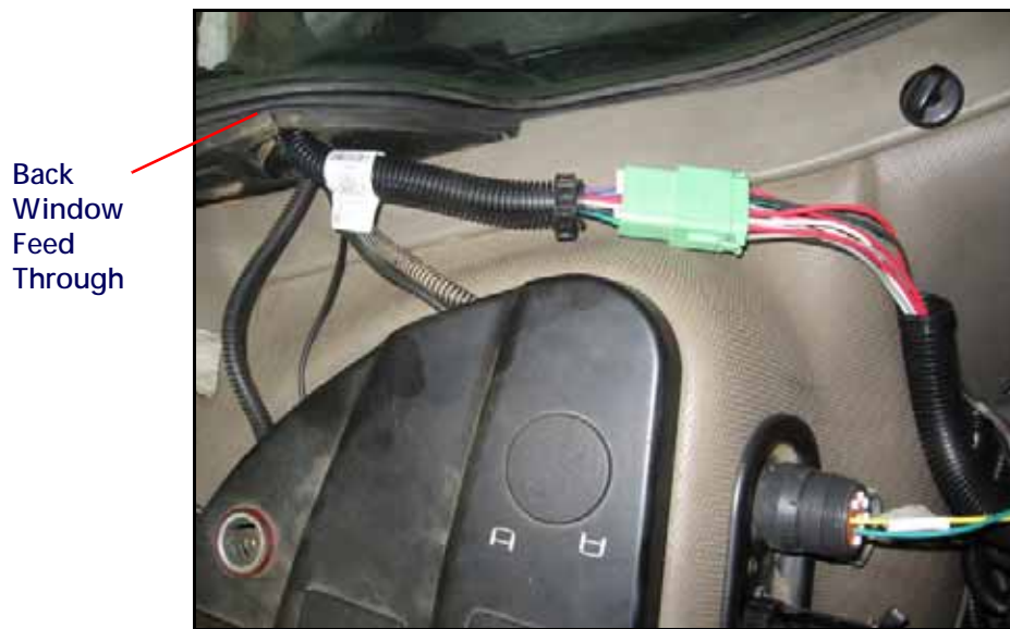
FIGURE 9. Feed Through in Back Window
