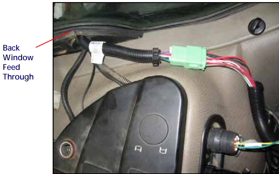
FIGURE 5. Feed Through in Back Window
