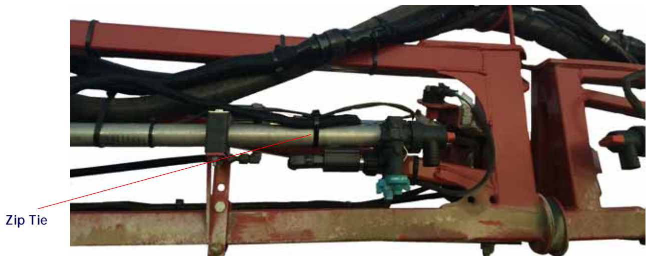
FIGURE 4. Securing Valve Branches
