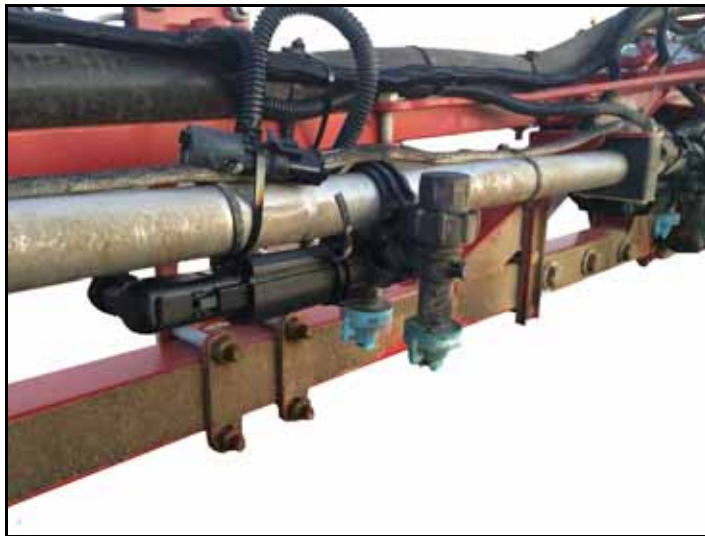
FIGURE 2. Modified Nozzle Control Valve Installation
