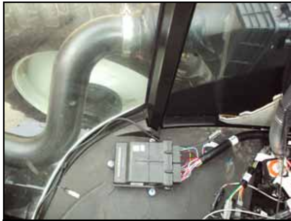
FIGURE 4. Node Harness Connected to the Node
