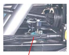
Hydraulic valve and pressure switch looking in from left side wheel well.
