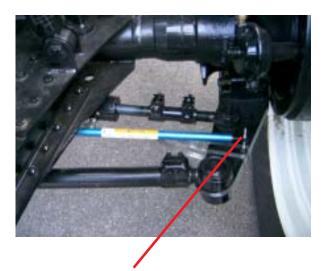
The other end of the wheel angle sensor is attached to the moving arm of the steering linkage using the provided band clamps, screw, and locknuts, and the mounting bracket.
