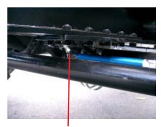
The wired end of the wheel angle sensor is attached to the right steering cylinder using band clamps, screw and lock-nuts, and the mounting bracket.
