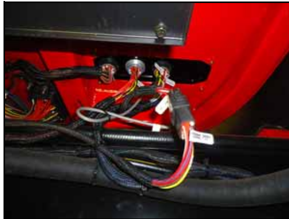
FIGURE 7. Valve Harness Connected to Bulkhead Plugs
