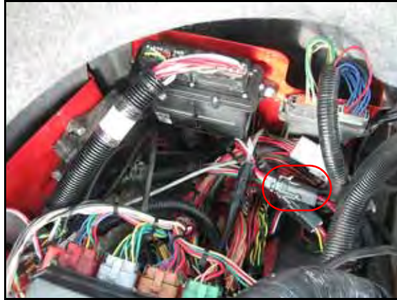
FIGURE 6. Node Harness Connected to Valve Harness
