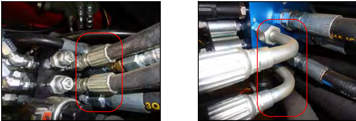
FIGURE 4. Left and Right Steering Hoses Installed
