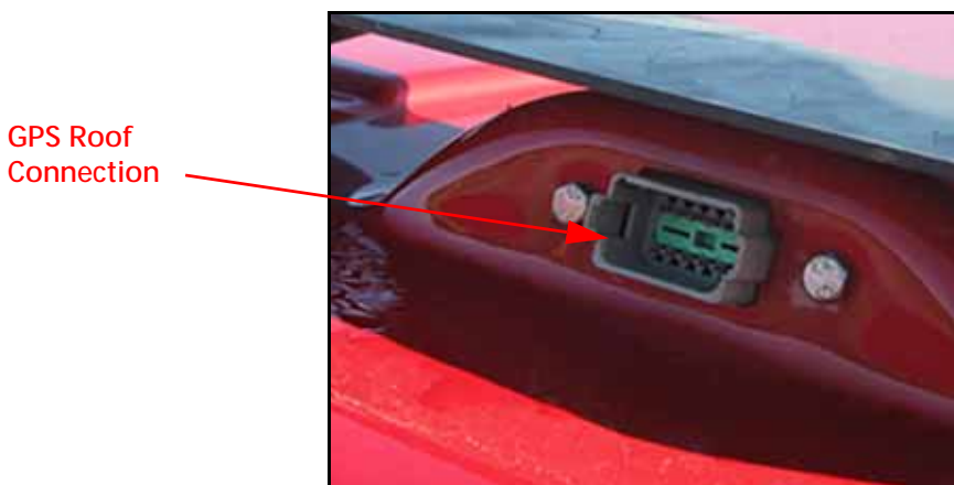
FIGURE 11. GPS Roof Connection
