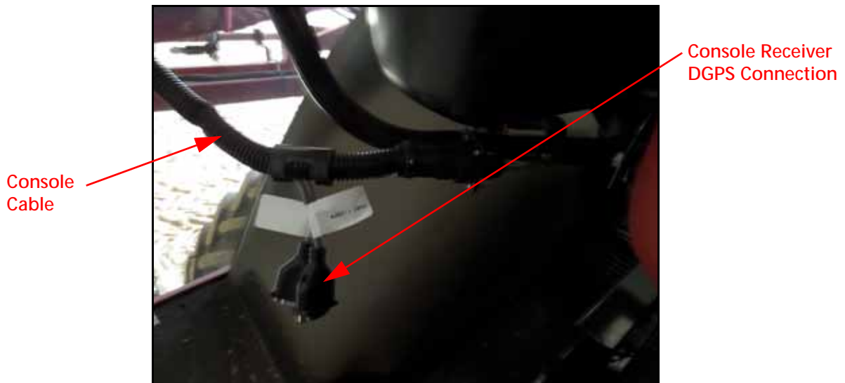
FIGURE 9. DGPS OUT Connected to Console Receiver Connection
