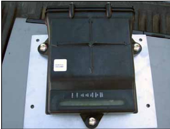
FIGURE 4. Node Installed on Mounting Plate
