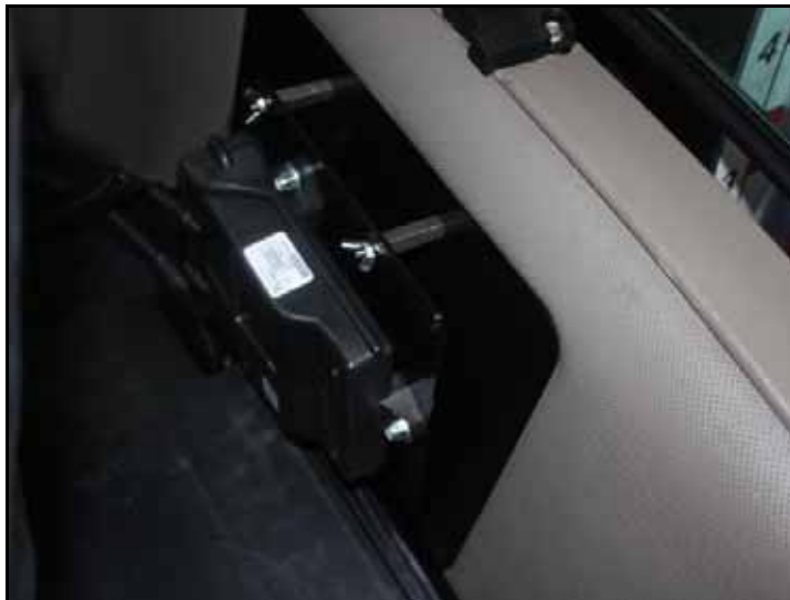
FIGURE 5. Node Plate Installed on Panel
