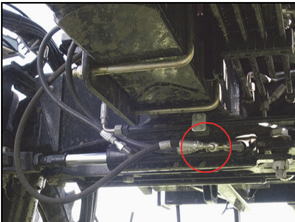
FIGURE 10. Right Steering Hose Installed
