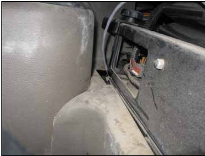
FIGURE 13. DGPS OUT Connector Routed Under Operator's Seat
