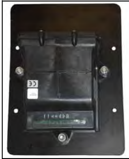
FIGURE 1. Node Mounted to the Mounting Plate
