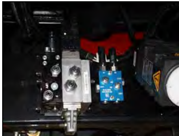
FIGURE 5. SmarTrax Valve Mounted on the Machine
