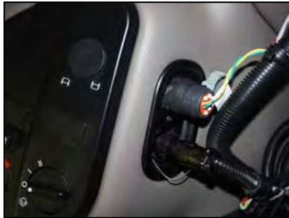
FIGURE 6. CAN Connector Installed on Machine's CAN System
