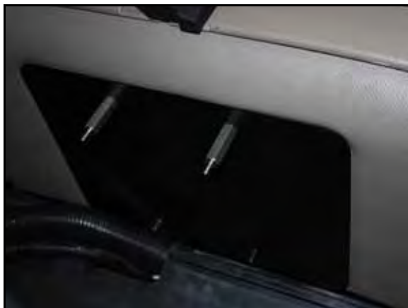
FIGURE 2. Standoffs Installed on Mounting Plate
