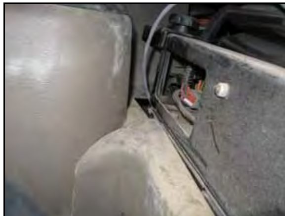
FIGURE 7. DGPS OUT Connector Routed Under Operator's Seat
