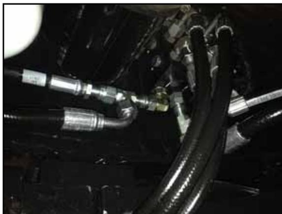
3. Install a -8 ORFS M/M/F swivel run tee adapter fitting (P/N 333-0012-028) on the machine's hydraulic block.
