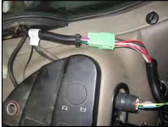
1. Route the valve cable through the right-rear corner cable access grommet under the window.
