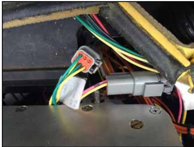
4. Connect the CAN adapter cable to the machine's X-7F connector.
