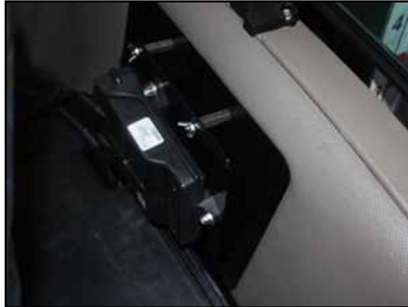
4. Mount the node mounting plate on the installed standoffs and secure with the machine's existing nuts that were previously removed.
