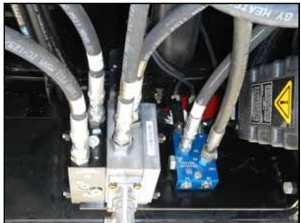
4. Install a -8 ORFS M/M/F swivel run tee adapter fitting (P/N 333-0012-028) on the hydraulic block.
