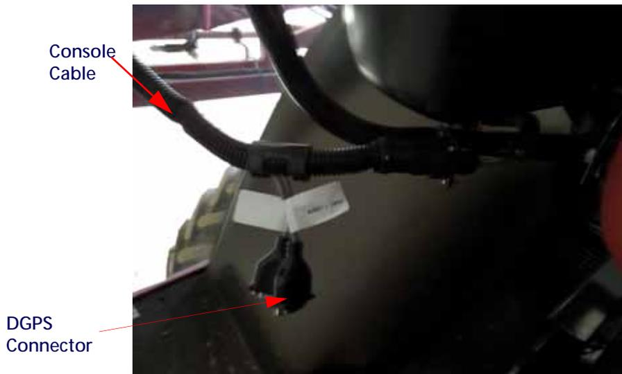
9. Connect the DGPS OUT connector to the Field computer cable's DGPS connection.
