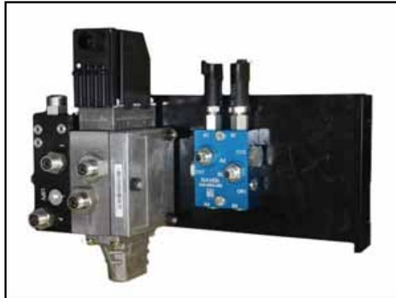
2. Mount the SmarTrax valve (P/N 334-0003-088) to the hydraulic valve mounting bracket (P/N 107-0172-534) using four 5/16" hex bolts (P/N 311-0052-104) and four 5/16" lock washers (P/N 313-1000-019).
