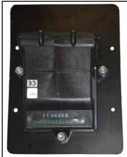
1. Mount the SmarTrax node (P/N 063-0173-228) to the node mounting plate (P/N 107-0172-084) using three 3/8" - 16 UNC nylon insert lock nuts (P/N 312-4000-061).
