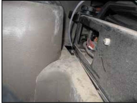
8. Route the DGPS OUT connector out the right corner of the operator's seat base and under the right arm rest.
