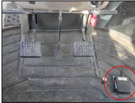
1. Select a suitable location for the foot switch (P/N 063-0172-470) to be installed.
