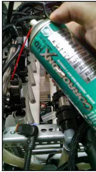
Applying Corrosion Inhibitor
