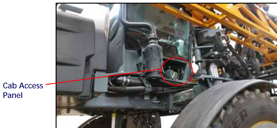
FIGURE 1. Exterior Cab Access Panel Removed
