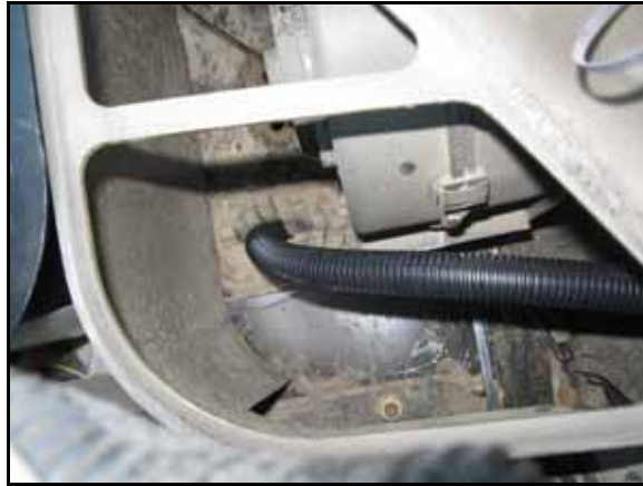
FIGURE 21. Valve Cable Routed Through Access Point
