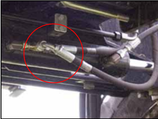
FIGURE 7. Installed Left Steering Hose
