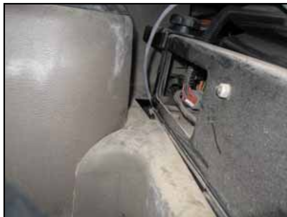
FIGURE 7. DGPS OUT Connector Routed Under Operator's Seat
