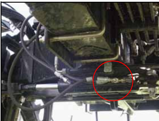
FIGURE 8. Installed Right Steering Hose
