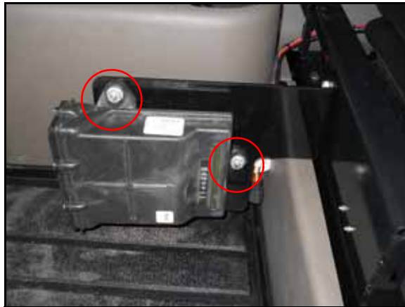
FIGURE 13. Node Installed on Mounting Bracket
