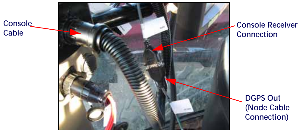
FIGURE 19. DGPS OUT Connected to Console Receiver Connection
