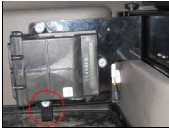
FIGURE 14. Node Support Bracket Secured to Node Mounting Bracket
