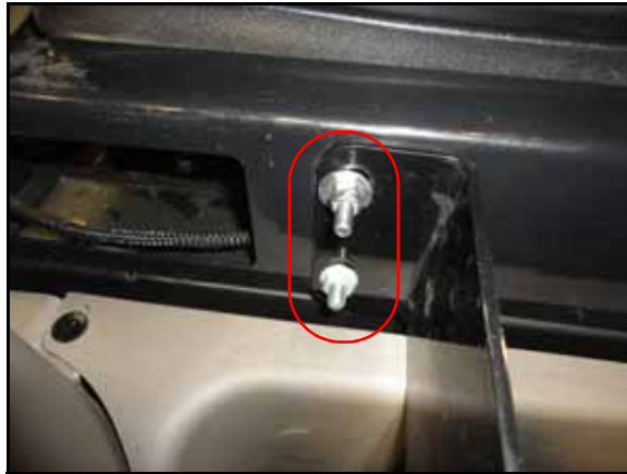
FIGURE 12. Node Mounting Bracket Installed
