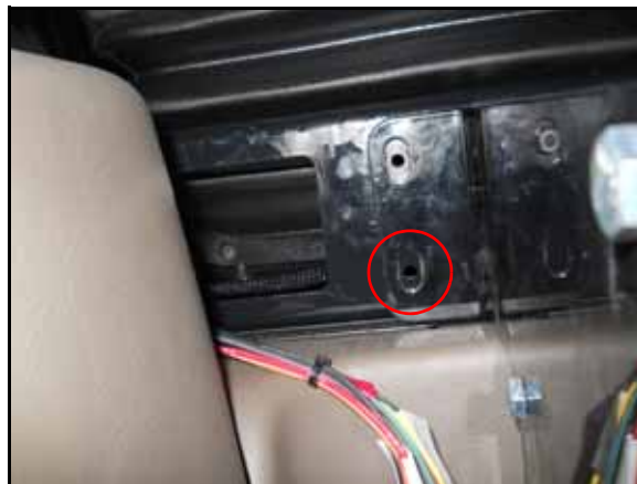
FIGURE 11. Hole Drilled in Machine's Bracket
