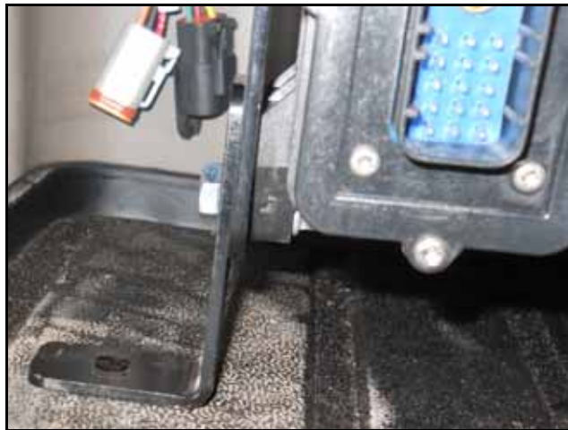
FIGURE 14. Node Support Bracket Secured to Cab Floor
