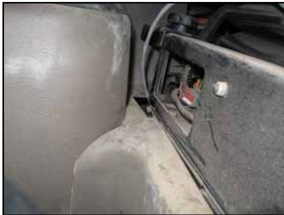
FIGURE 6. DGPS OUT Connector Routed Under Operator's Seat
