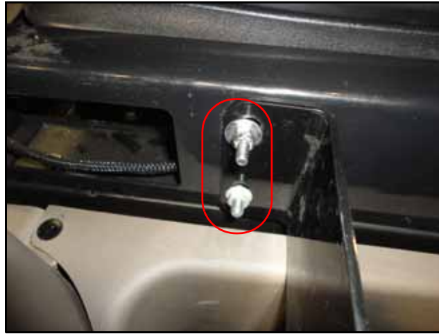
FIGURE 11. Node Mounting Bracket Installed
