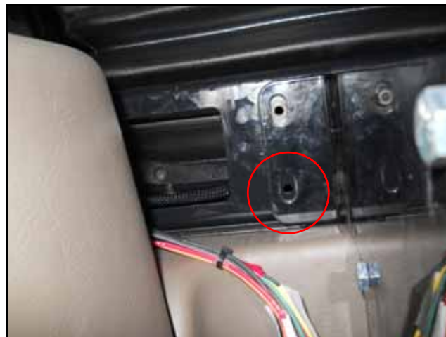
FIGURE 10. Hole Drilled in Machine's Bracket
