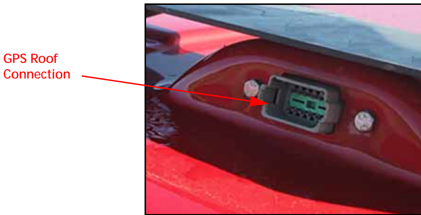
FIGURE 22. GPS Roof Connection
