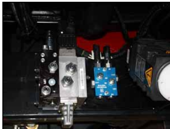
FIGURE 5. SmarTrax Valve Mounted on the Machine
