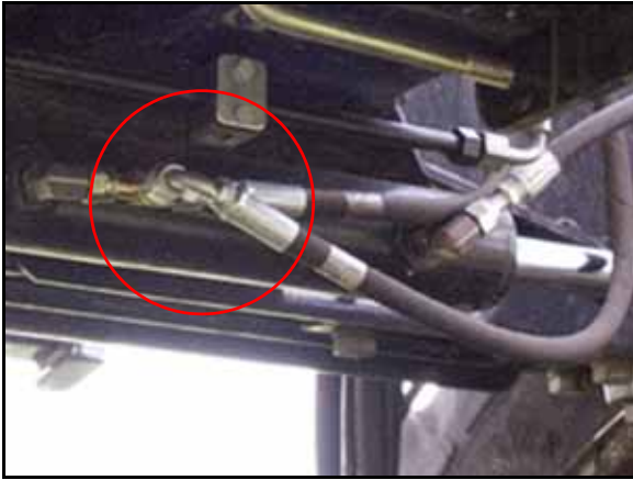
FIGURE 8. Installed Left Steering Hose
