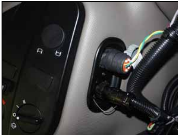
FIGURE 6. CAN Connector Installed on Machine's CAN System
