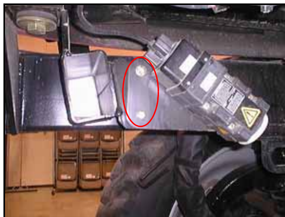
FIGURE 3. Mounting Bracket Installed
