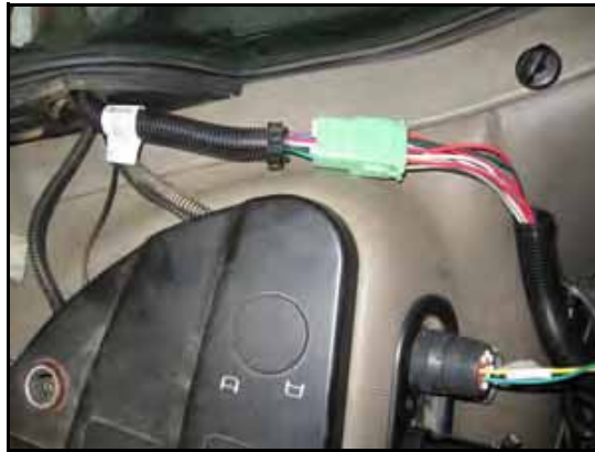
FIGURE 10. Valve Cable Routed Through Access Point
