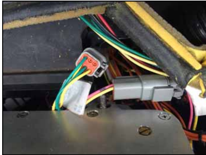
FIGURE 7. CAN Connector Installed on Machine's CAN System
