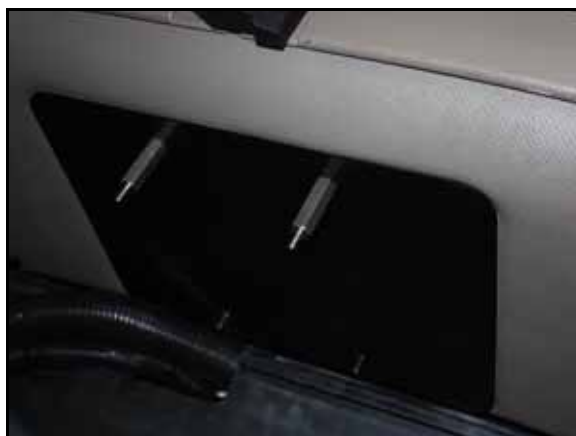
FIGURE 2. Standoffs Installed on Mounting Plate
