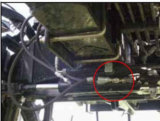
FIGURE 9. Installed Right Steering Hose
