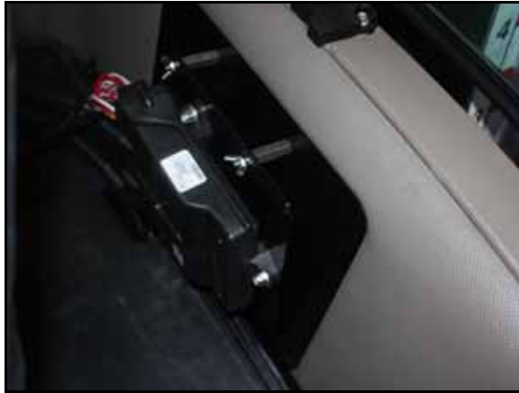
FIGURE 5. Node Cable Installed on Node
