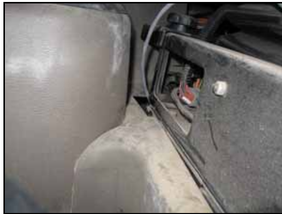
FIGURE 8. DGPS OUT Connector Routed Under Operator's Seat
