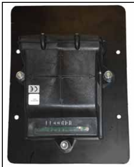
FIGURE 1. Node Mounted to the Mounting Plate
