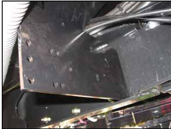
FIGURE 4. Mounting Bracket Installed on Left Frame Rail (Beside Radar)
