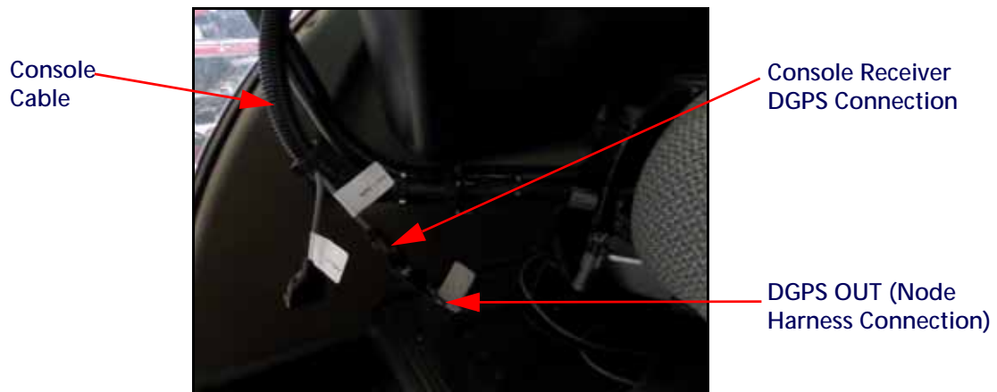
FIGURE 7. DGPS OUT Connected to Console Receiver Connection
