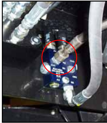
FIGURE 6. Machine's Left Steering Hose Installed on Flow Switch
