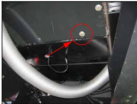
FIGURE 3. New Air Cleaner Hose Mounting Clamp Location
