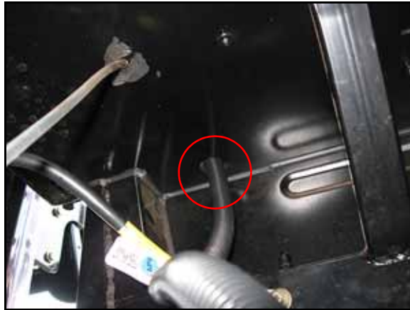
FIGURE 10. Valve Harness Routed into the Cab
