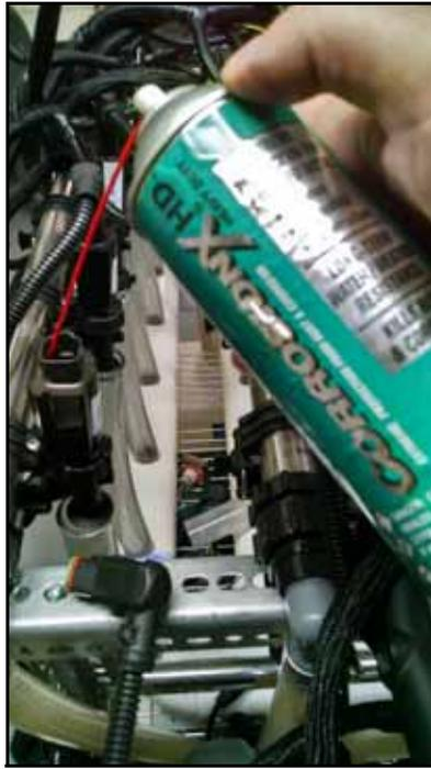
Corrosion Inhibitor Applied
