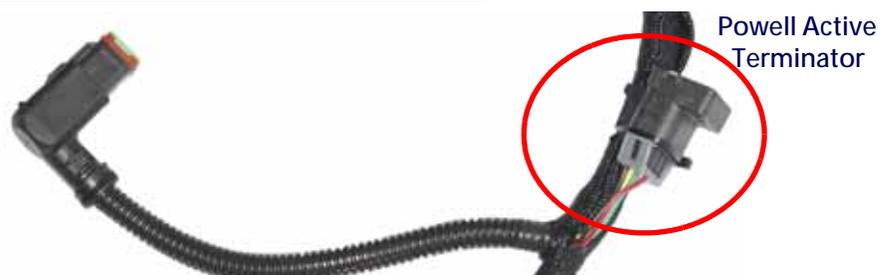
2. Verify the terminator is tightly secured to the main cable harness with a zip tie. If the terminator is not secured, excessive stress on the wires can cause breakage and intermittent nozzle CAN communication.
