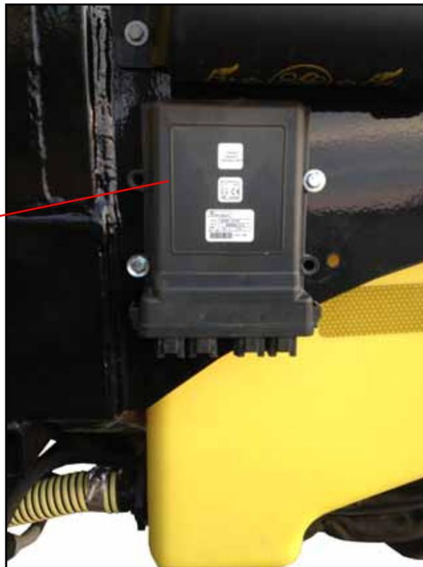
2. Secure the Product Controller II to the mounting bracket using the four bolts, four nuts, and eight washers (provided).
