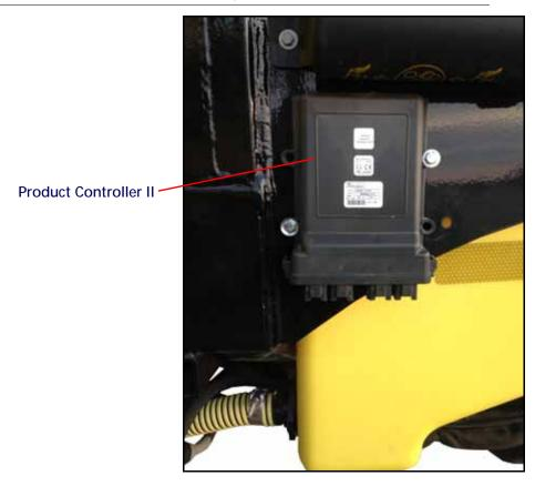
2. Secure the Product Controller II to the mounting bracket using the four bolts, four nuts, and eight washers (provided).
