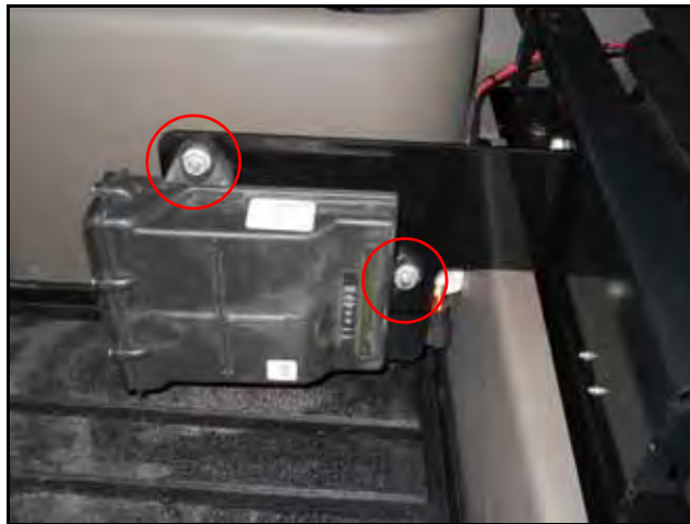
FIGURE 13. Node Installed on Mounting Bracket
