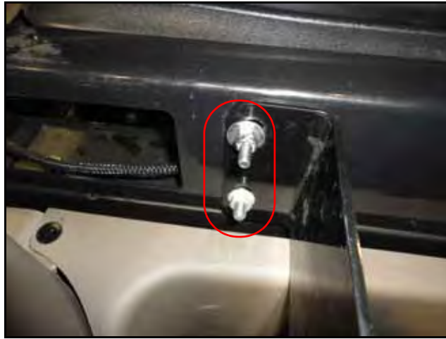
FIGURE 12. Node Mounting Bracket Installed
