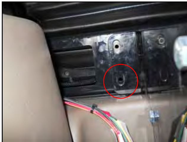
FIGURE 11. Hole Drilled in Machine's Bracket
