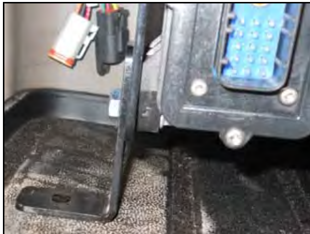
FIGURE 15. Node Support Bracket Secured to Cab Floor
