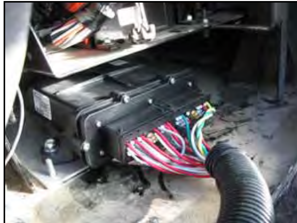
FIGURE 6. Node Harness Installed on Node
