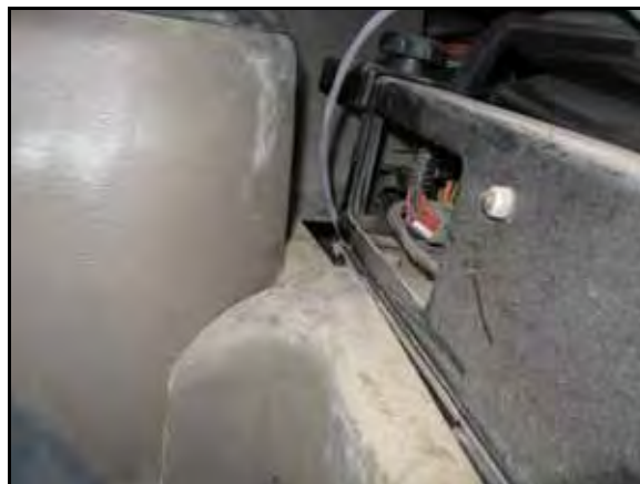
FIGURE 7. DGPS OUT Connector Routed Under Operator's Seat
