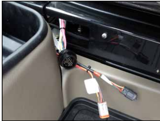
FIGURE 18. Convenience Tray Removed
