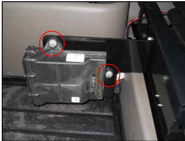
FIGURE 13. Node Installed on Mounting Bracket
