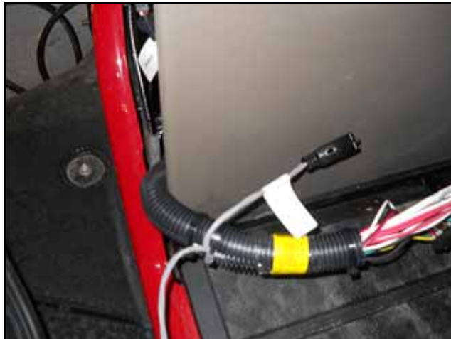
FIGURE 17. Node Harness Routing
