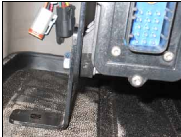
FIGURE 15. Node Support Bracket Secured to Cab Floor
