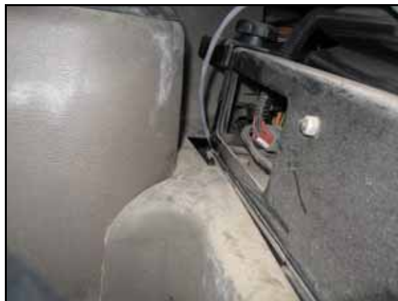
FIGURE 7. DGPS OUT Connector Routed Under Operator's Seat
