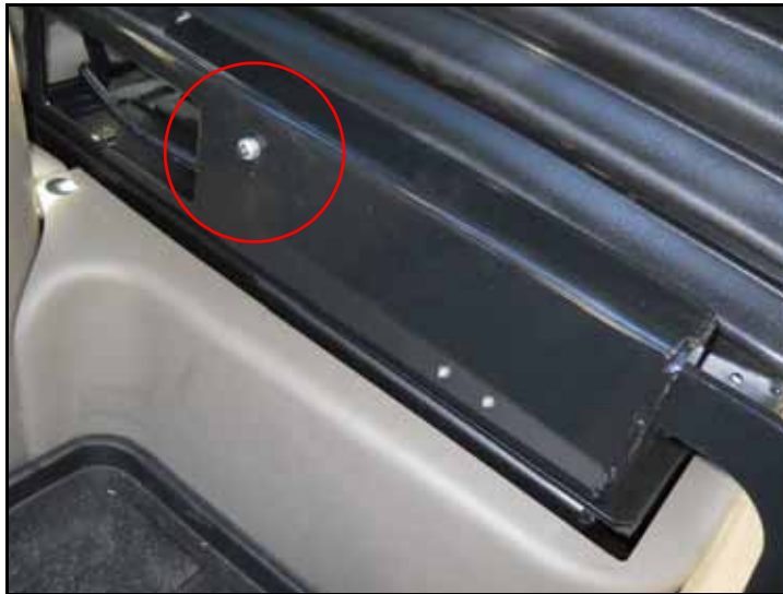
FIGURE 10. Node Mounting Location
