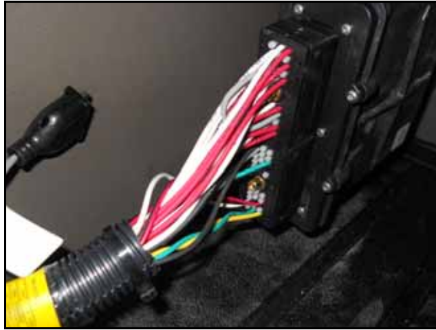
FIGURE 16. Node Harness Installed on Node
