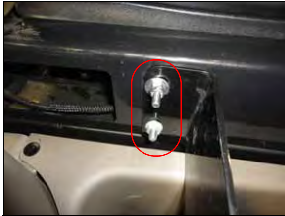
FIGURE 12. Node Mounting Bracket Installed
