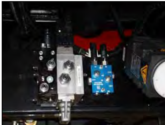
FIGURE 5. SmarTrax Valve Installed on Mounting Bracket
