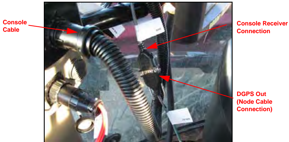
FIGURE 9. DGPS OUT Connected to Console Receiver Connection
