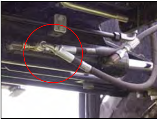
FIGURE 8. Installed Left Steering Hose
