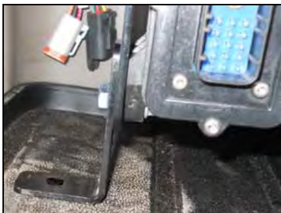
FIGURE 15. Node Support Bracket Secured to Cab Floor
