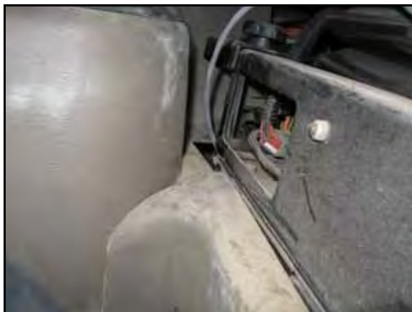
FIGURE 7. DGPS OUT Connector Routed Under Operator's Seat
