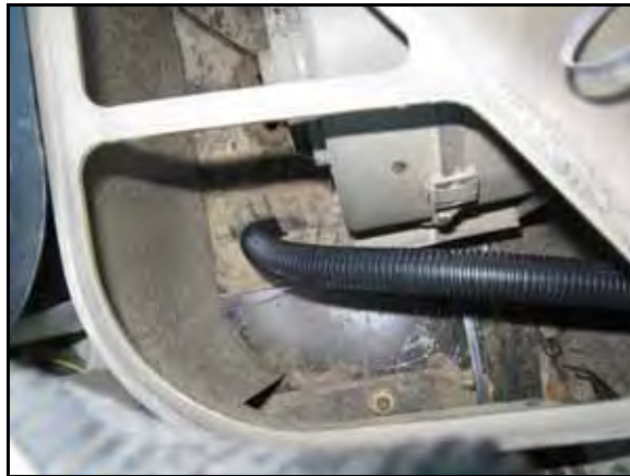
FIGURE 21. Valve Cable Routed Through Access Point
