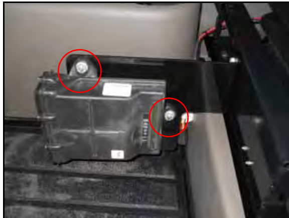
FIGURE 13. Node Installed on Mounting Bracket
