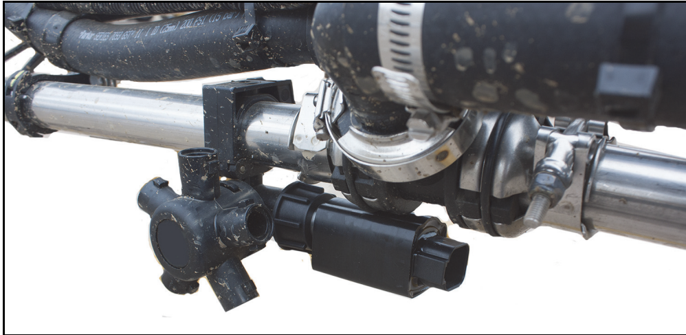
FIGURE 3. Modified Nozzle Control Valve Installation
