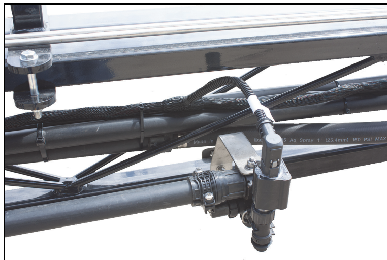
FIGURE 4. Securing Valve Branches
