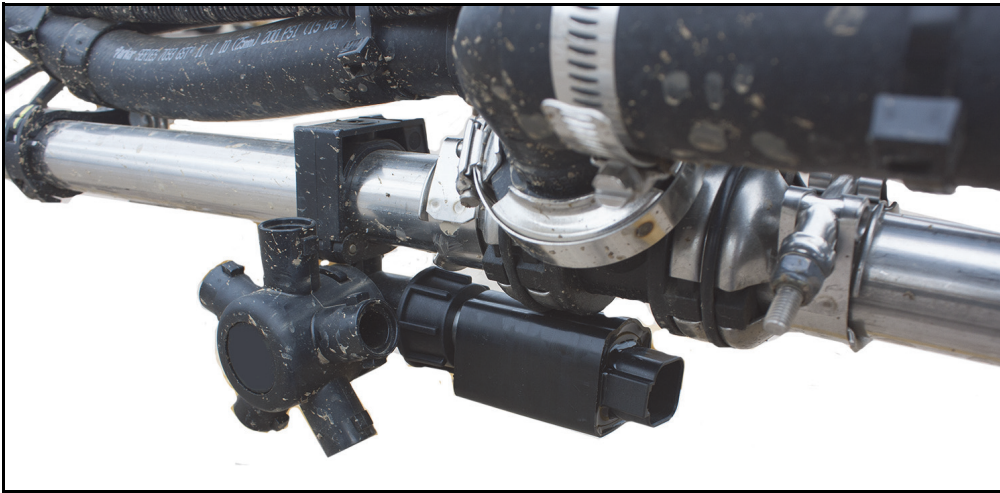
FIGURE 2. Modified Nozzle Control Valve Installation
