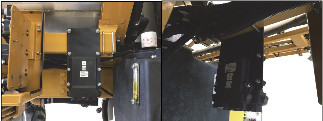
FIGURE 4. Completed ECU Installation
