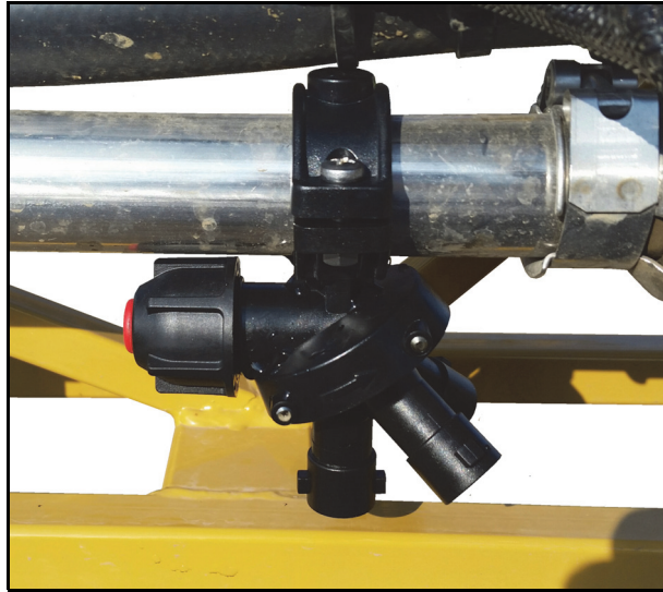
FIGURE 4. Triple Nozzle Body Installed
