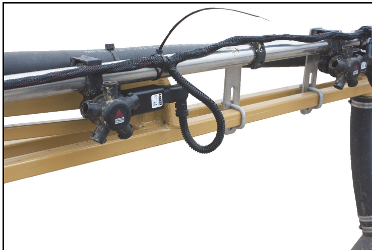
FIGURE 6. Securing Valve Branches
