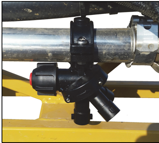
FIGURE 4. Triple Nozzle Body Installed
