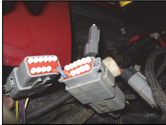
FIGURE 12. Fence Row Adapter Cable Installed
