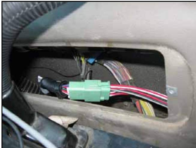
FIGURE 21. Valve Harness Connected to Node Harness
