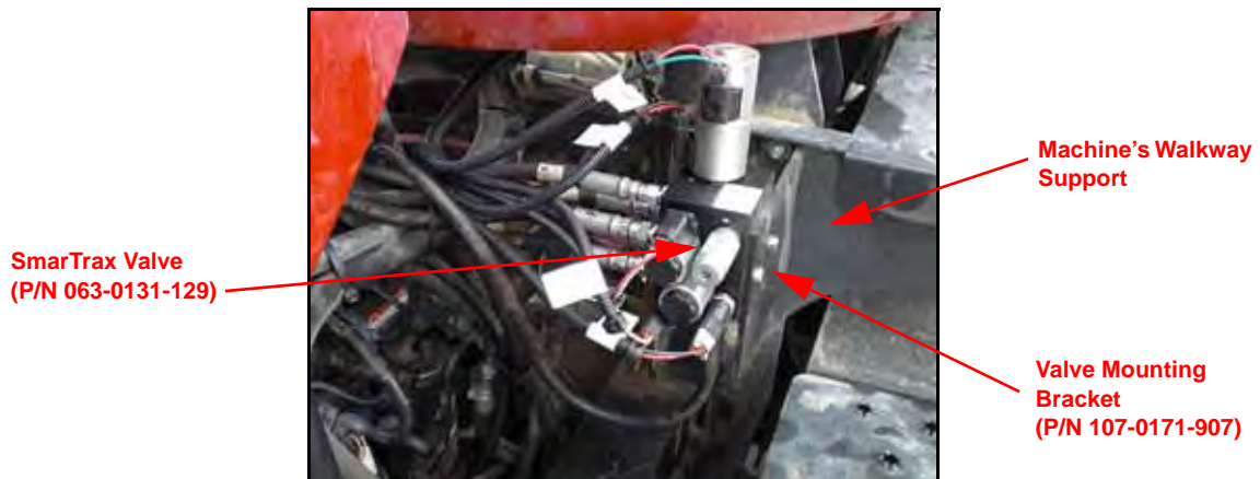
FIGURE 3. SmarTrax Valve Mounted to the Machine
