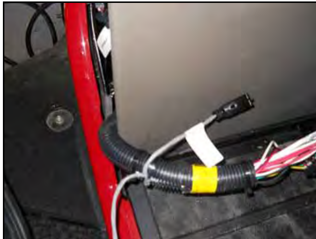
FIGURE 17. Node Harness Routing
