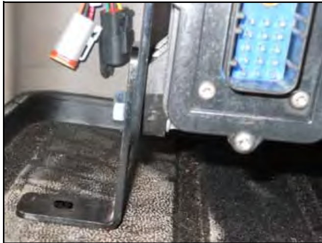
FIGURE 15. Node Support Bracket Secured to Cab Floor
