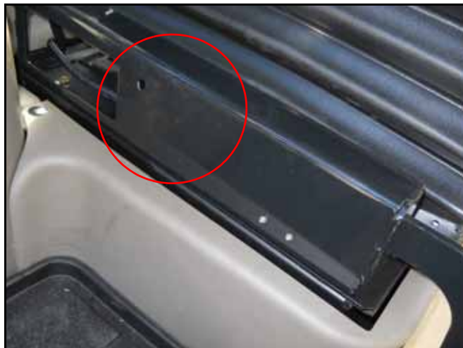
FIGURE 10. Node Mounting Location
