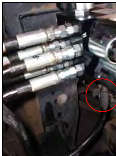
FIGURE 13. SmarTrax Valve LS STEER Hose Connections
