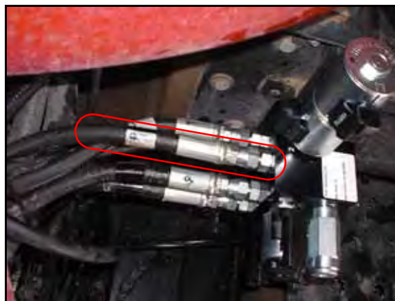
FIGURE 9. Pressure Hose Installed on SmarTrax Valve
