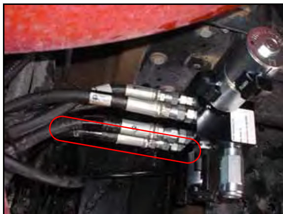
FIGURE 7. Right Steering Hose Installed on SmarTrax Valve
