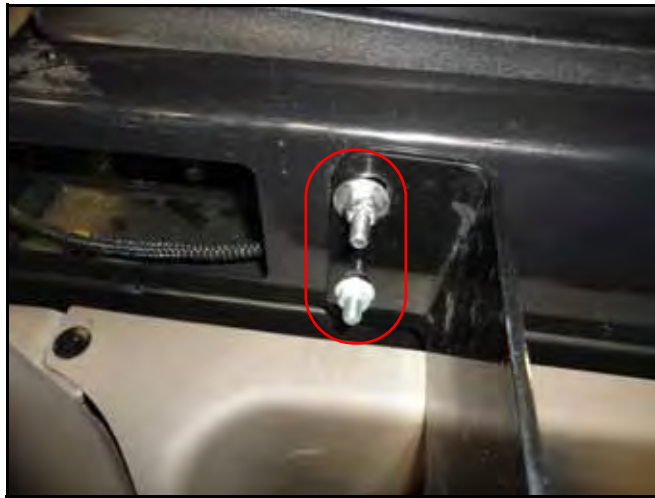
FIGURE 12. Node Mounting Bracket Installed
