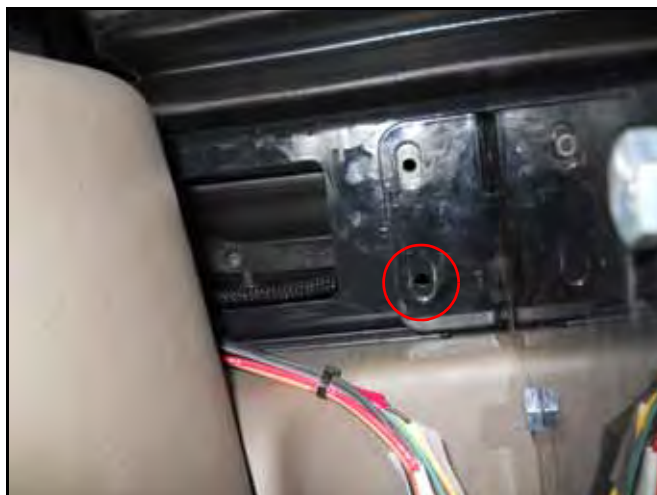
FIGURE 11. Hole Drilled in Machine's Bracket
