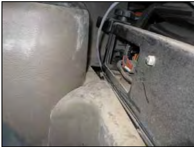
FIGURE 7. DGPS OUT Connector Routed Under Operator's Seat
