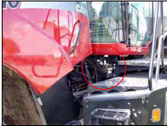
FIGURE 2. SmarTrax Valve Mounting Location
