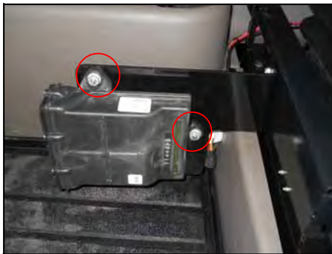
FIGURE 13. Node Installed on Mounting Bracket
