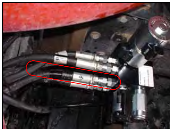
FIGURE 5. Left Steering Hose Installed on SmarTrax Valve
