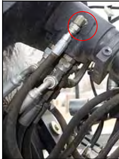
FIGURE 12. Load Sense Port on the Steering Orbital
