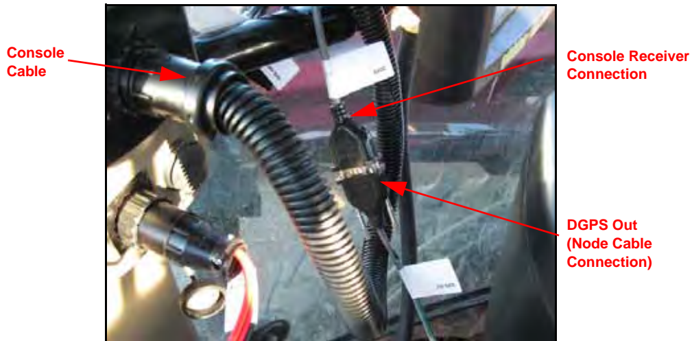
FIGURE 9. DGPS OUT Connected to Console Receiver Connection
