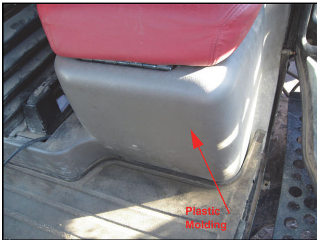
FIGURE 3. Removing Instructional Seat Molding
