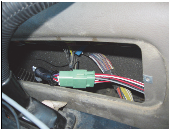
FIGURE 14. Valve Harness Connected to Node Harness
