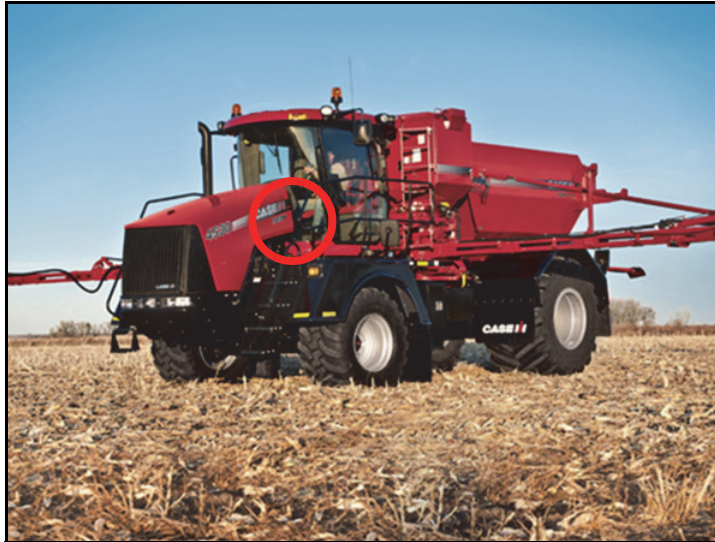
FIGURE 2. SmarTrax Valve Mounting Location
