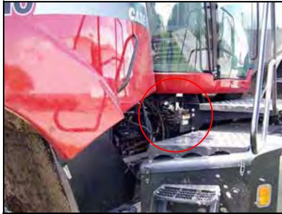
FIGURE 2. SmarTrax Valve Mounting Location
