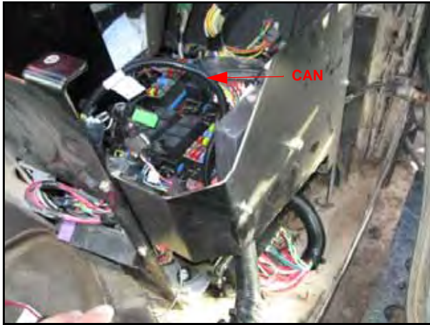
FIGURE 9. CAN Connector Installed on Machine's CAN System
