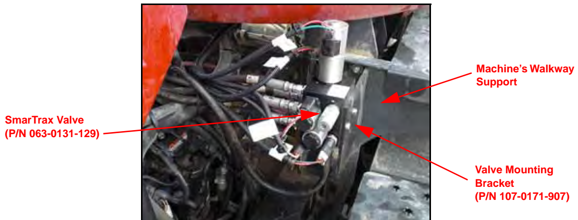
FIGURE 3. SmarTrax Valve Mounted to the Machine
