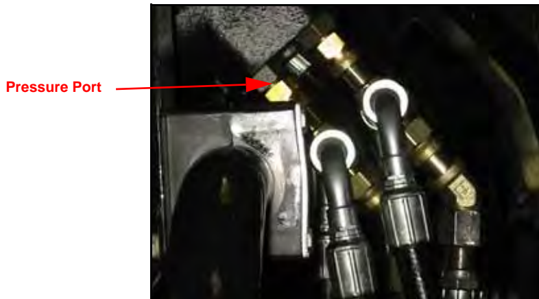
FIGURE 8. Pressure Hose Installed
