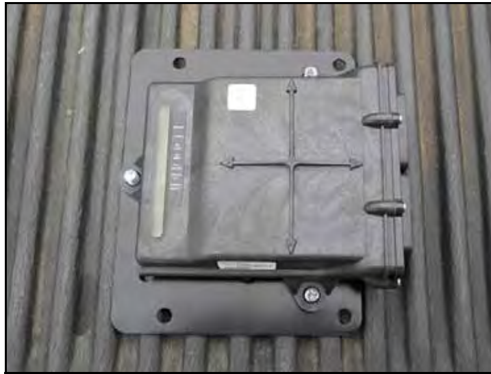
FIGURE 4. Node Mounted to Mounting Plate
