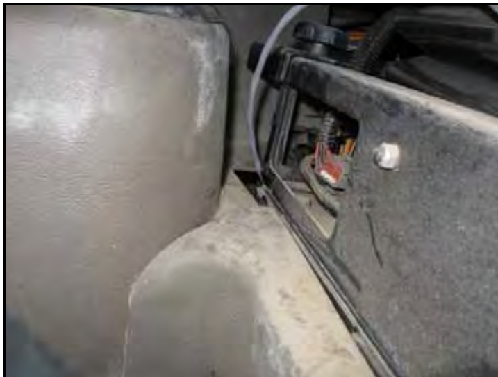
FIGURE 10. DGPS OUT Connector Routed Under Operator's Seat
