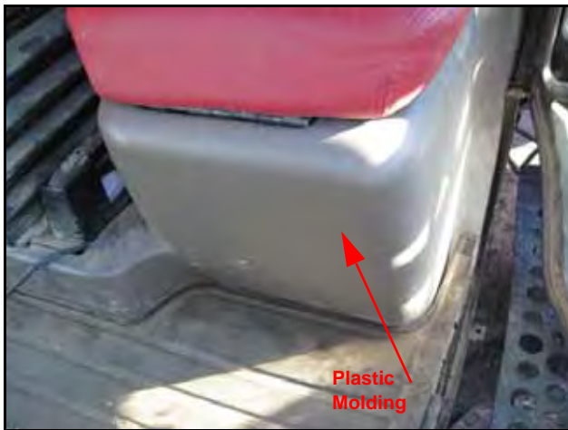
FIGURE 3. Removing Instructional Seat Molding
