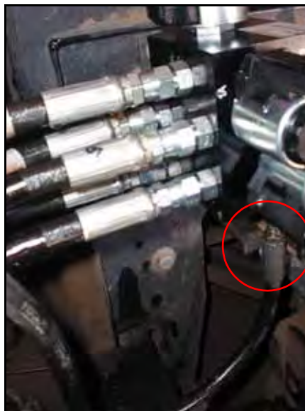
FIGURE 13. SmarTrax Valve LS STEER Hose Connections
