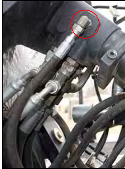
FIGURE 12. Load Sense Port on the Steering Orbital
