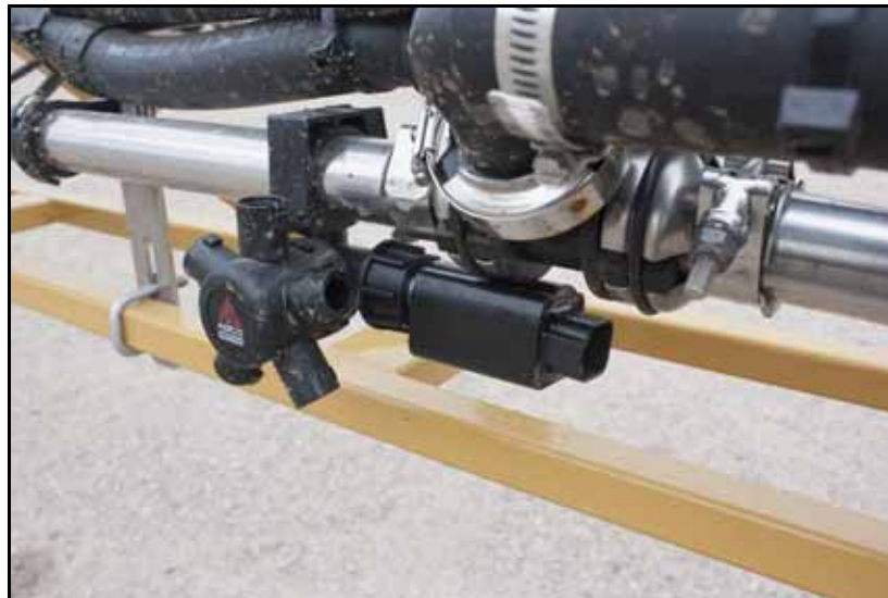
FIGURE 3. Modified Nozzle Control Valve Installation
