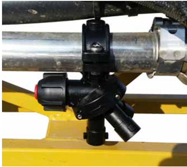
FIGURE 4. Triple Nozzle Body Installed
