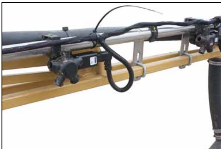
FIGURE 6. Securing Valve Branches
