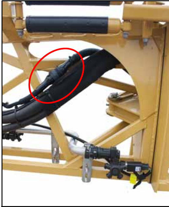
FIGURE 7. Primary and Secondary Boom Cable Connection at Mid-Boom Fold Point
