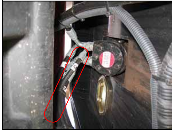
FIGURE 4. Machine's Existing Load Sense Hose
