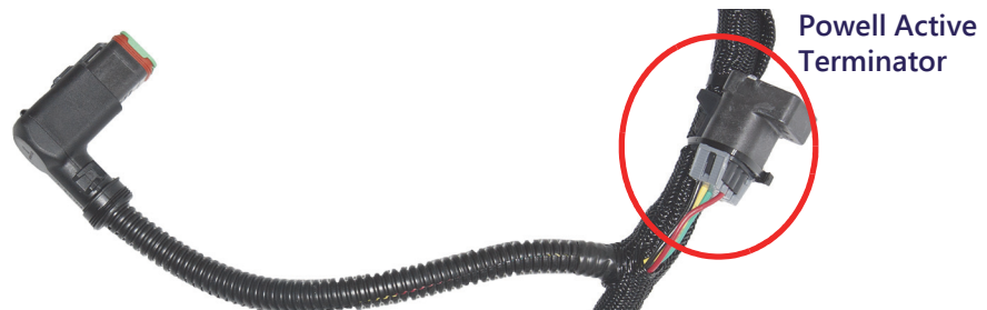
FIGURE 5. Secondary Cable ISOBUS Powell Terminator
