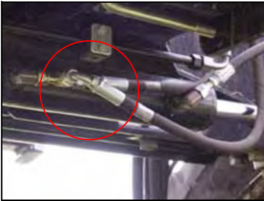
FIGURE 8. Installed Left Steering Hose
