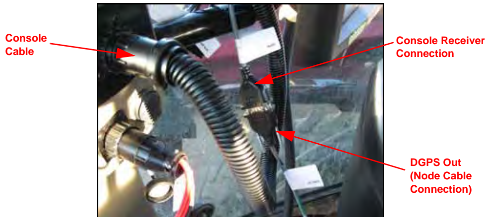
FIGURE 10. DGPS OUT Connected to Console Receiver Connection
