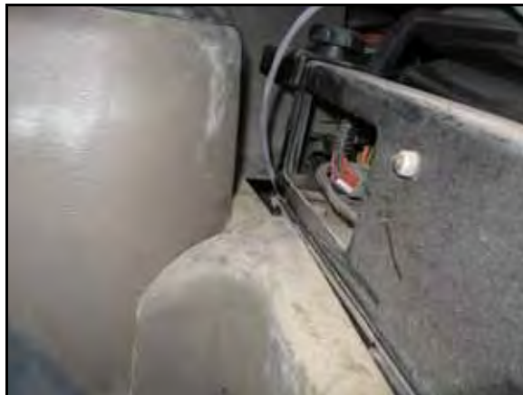
FIGURE 9. DGPS OUT Connector Routed Under Operator's Seat
