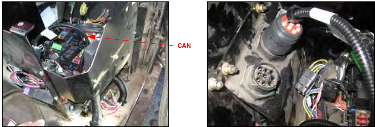
FIGURE 8. CAN Connector Installed on Machine's CAN System
