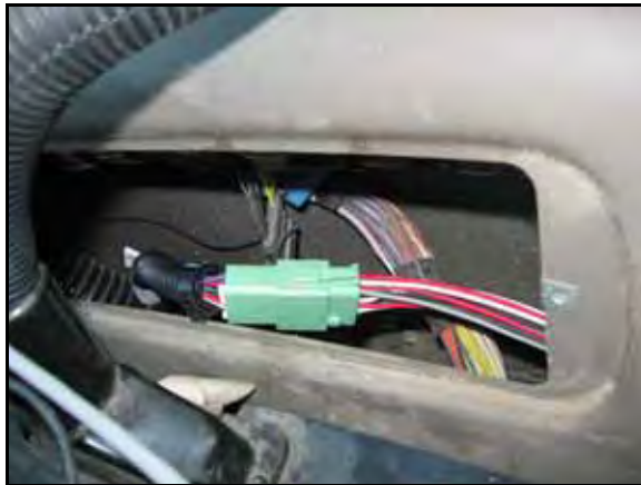
FIGURE 13. Valve Cable Connected to Node Cable
