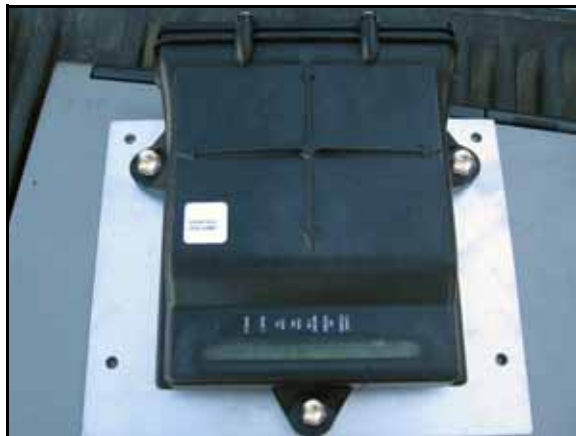
FIGURE 4. Node Mounted to Mounting Plate
