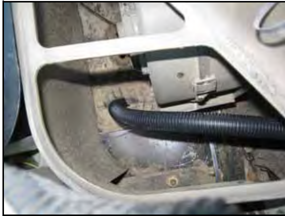
FIGURE 12. Valve Cable Routed Through Access Point
