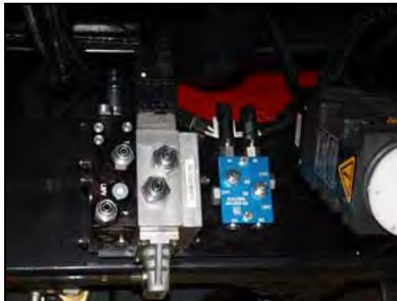
FIGURE 5. SmarTrax Valve Installed on Mounting Bracket
