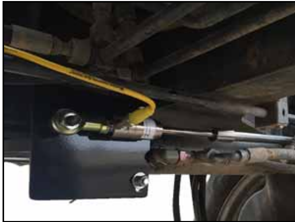
FIGURE 6. Base-End of WAS Installed on Base-End of Steering Cylinder
