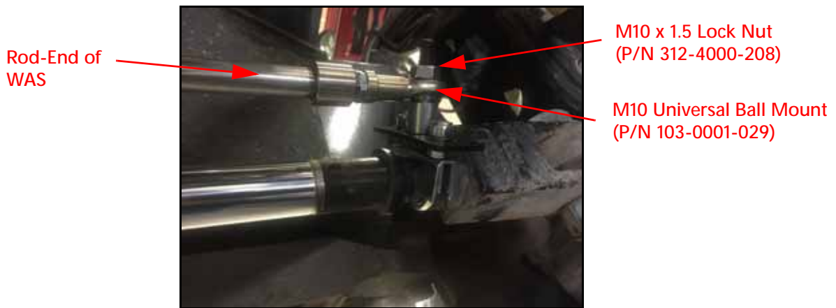
FIGURE 5. Rod-End of WAS Installed on Rod-End of Steering Cylinder
