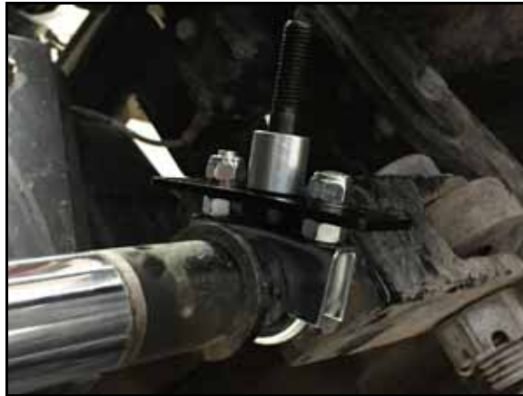
FIGURE 4. Small WAS Mounting Bracket Installed on Rod-End of Steering Cylinder
