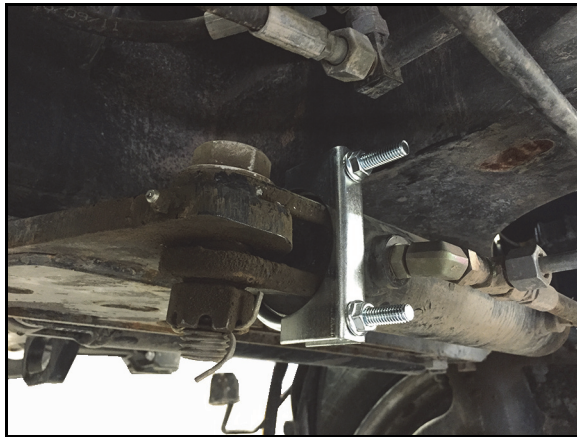
FIGURE 2. Muffler Clamp Installed on Steering Cylinder
