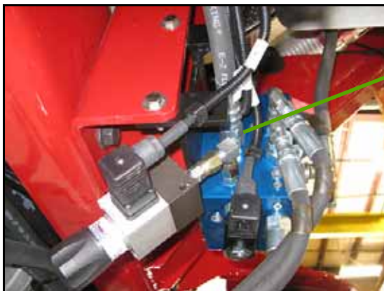
FIGURE 2. SmarTrax Block Hydraulic Connections
