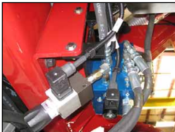
FIGURE 6. Steering Override Pressure Switch
