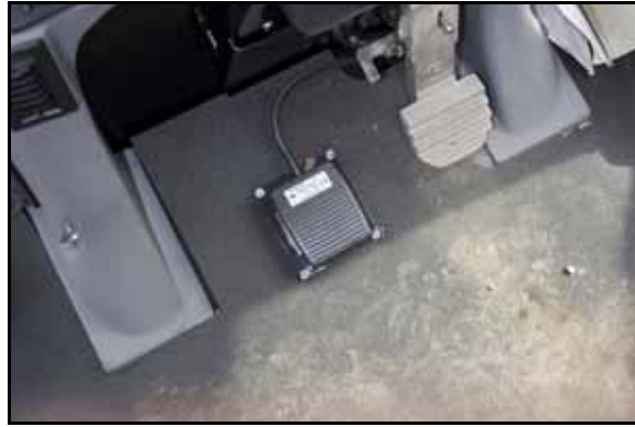
FIGURE 3. Foot Switch Mounting Example
