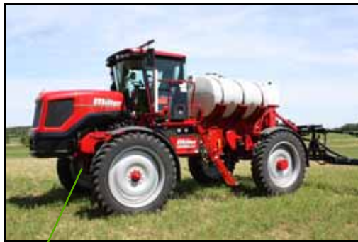
SmarTrax Hydraulic Valve Mounting Location (Right Side of Machine)
