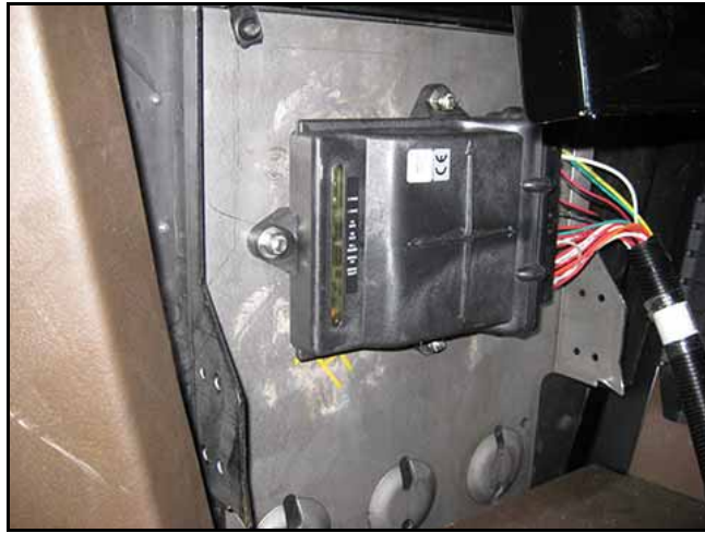
FIGURE 5. SmarTrax Node Mounting Location
