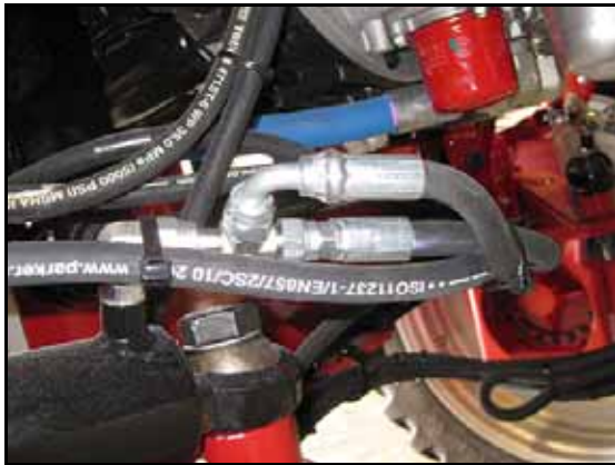
FIGURE 5. Steering Cylinder Connections
