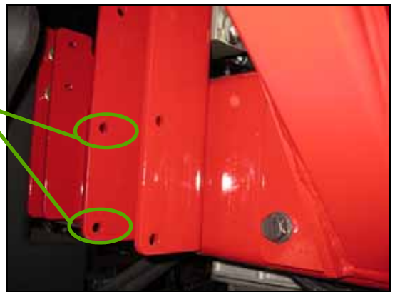
SmarTrax Hydraulic Valve Mounting Location
