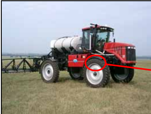
SmarTrax Hydraulic valve mounting location
