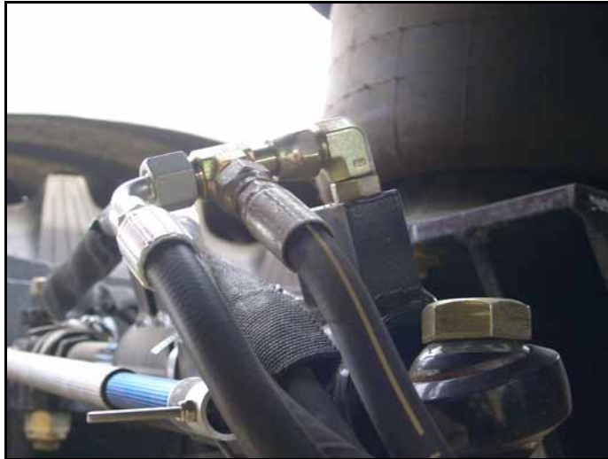
FIGURE 5. Steering Cylinder Connections
