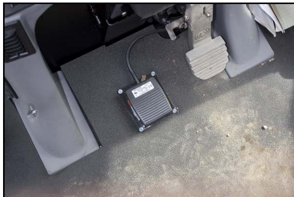
FIGURE 1. Foot Switch Mounting Example
