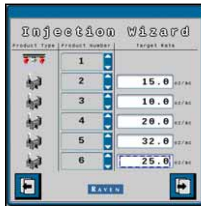
FIGURE 2. Product Controller II ECU Desired Target Rate
