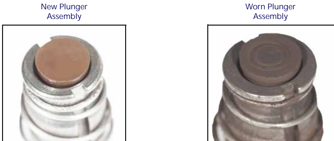
FIGURE 4. Plunger Inspection Detail
