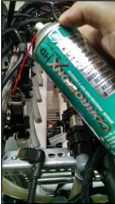
FIGURE 1. Applying Corrosion Inhibitor
