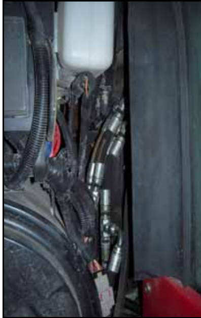
FIGURE 2. Supplied Hoses Installed on the Machine's Steering Orbitrol
